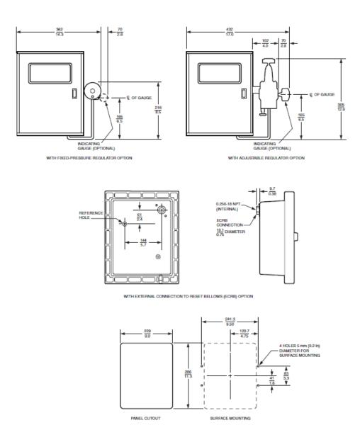
For horizontal multiple panel mounting, a minimum distance of 267 mm (10.5 in.) from center line to center line is required. For vertical multiple panel mounting, a minimum distance of 375 mm (14.8 in.) from center line to center line is required.
